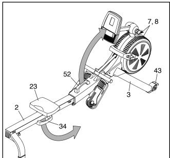
Next, hold and lift the Frame Handle (52) and the Rail Handle (34), and tip the rower forward onto the Shields (7, 8) and the Storage Feet (43).
